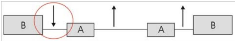
With **Link Loss Forwarding**, a link down (↓) detected on the Ethernet port will force a link down on the fiber port and vice-versa. The up link (↑) will stop transmitting and turn "off" as soon as the remote link is down.
