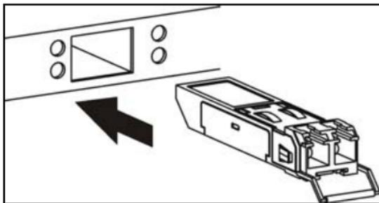
SFP transceiver module installation orientation varies depending on your device. Your SFP transceiver module comes with a mechanism that prevents incorrect insertion.
