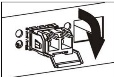
5. Using your thumb and index finger, grasp the tabs on both sides of the module and carefully slide it out of the slot.
