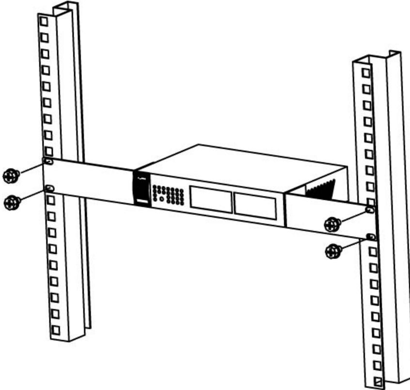
**Figure 9** Mounting the Switch on a Rack (ES1100-24)
