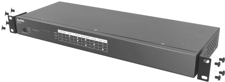
Figure 2 Attaching the Rack Mounting Brackets
