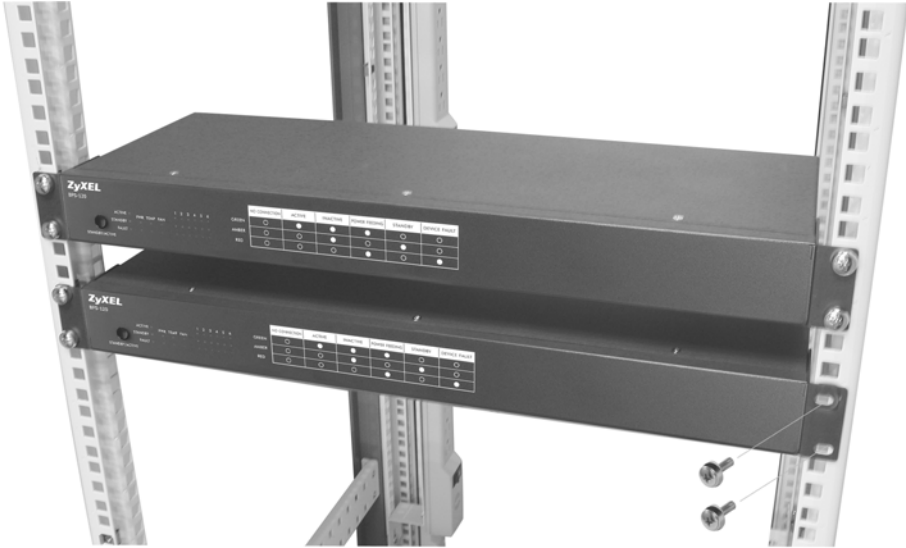
Figure 3 Rack Mounting the BPS-120
